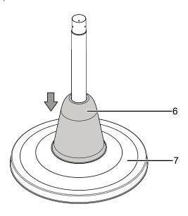
3. Screw together the foot (7), the central rod (4) and the telescopic rod with twist lock (3).
