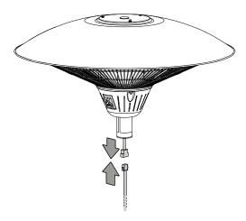
5. Guide the mains cable from above through the mounted rod and foot.
