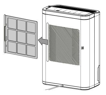
2. Clean the filter using a slightly damp, soft, lint-free cloth. If the filter is heavily contaminated, clean it with warm water mixed with a neutral cleaning agent.
