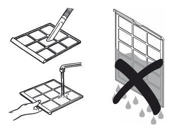
3. Allow the filter to dry completely. Do not insert a wet filter into the device!
